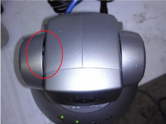
The gap cause the lose of holding power of the arms then cause the Pan-Tilt failed to move up/down.
