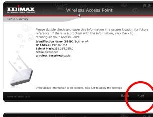
5. The device will save your settings, then reboot. Please do not disconnect or turn off the device during this process.
