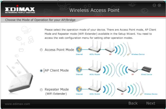
Access Point Mode is the default mode. We use one network cable to connect AP to a broadband router. Wireless devices will see the signal from Edimax AP and connect to Internet.
