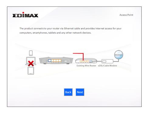
**2.** Connect the network port of your RG21S/RA21S to the LAN port of your existing router using an Ethernet cable, then click "Next".
